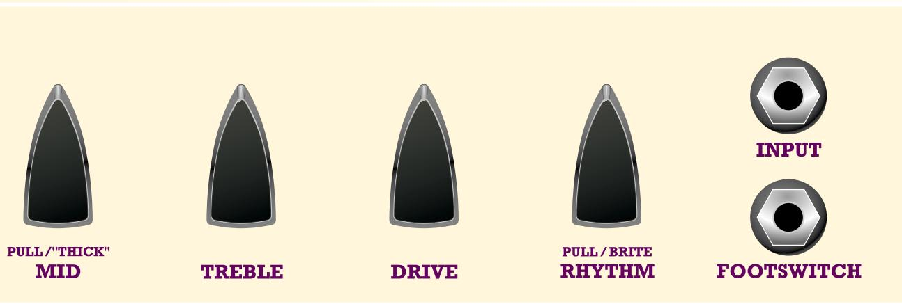
**Treble:** Use this control to dial in your treble frequencies. Typically, guitars that use single coils will require less treble and humbuckers more.
